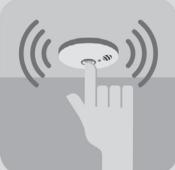
Push the test button to sound the smoke alarm.
